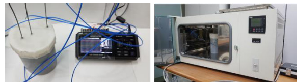
Fig. 2. Measuring the heat-generating temperature of the solidification depending on the curing temperature– Room temperature (L), 50℃ atmosphere (R).
