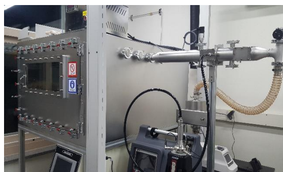
Fig. 2. The system for aerosol measurement from metal cutting in KAIST Nuclear Fuel Cycle Lab.
