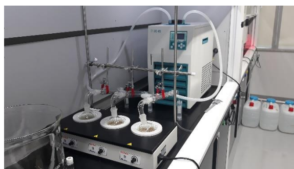
Fig. 2. Tritium Pretreatment (Heat Exchange Cooler).
