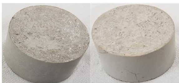
Fig. 1. Thermal treatment at 105°C (left) and 550°C (right).
