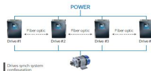
Fig. 1. Drives synch system configuration.
