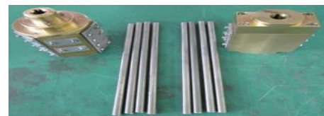
Fig. 2. Blade types and simulated fuel rods. (2-CUT module and 3-CUT module)
