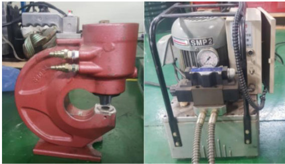
Fig. 2. Hydraulic punching machine and hydraulic pump.
