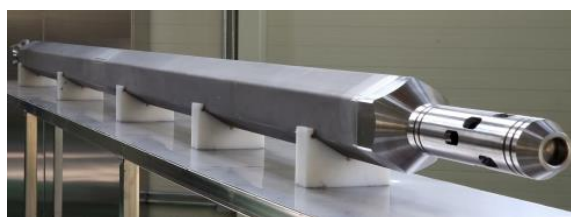
Fig. 1. Schematic view of fuel assembly for PGSFR.
