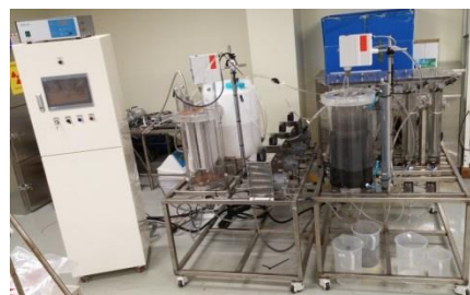
Fig. 2. Semi-Pilot decontamination system(4L/hr).
