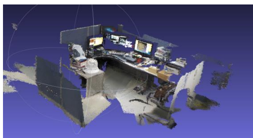
Fig. 3. Mapping of Desk Area using RTAB-Map.
