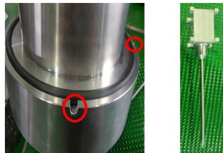
Fig. 2. O-ring holes and changing tool.
