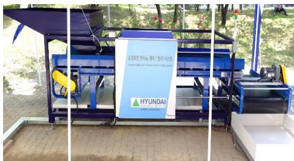
Fig. 2. Real-time measurement and segregation system.
