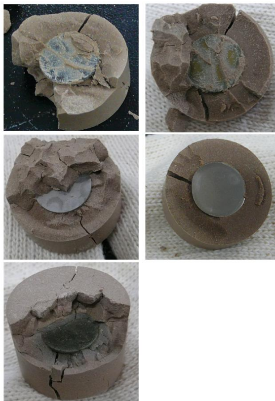
Fig. 2. The 3.2 year old test specimens with compact bentonite right after dismantling.
