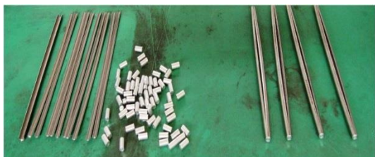
Fig. 5. Slitting shapes of 2-CUT and 3-CUT modules.
