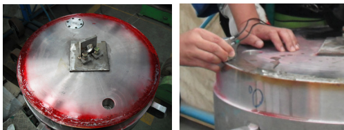
Fig. 2. LT(Left) and UT(Right) for SNF Canister drop test model.
