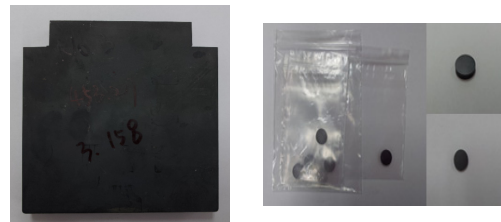
Fig. 1. SiC samples for the measurement of thermal diffusivity.
