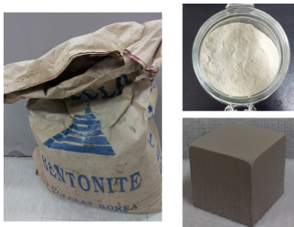
Fig. 1. GyeongJu bentonite powder and its compacted cubic block.
