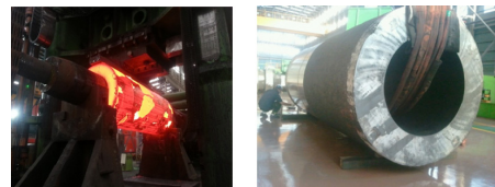
Fig. 4. Cask body forging.
