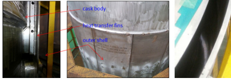
Fig. 7. Heat transfer fin and resin pouring.
