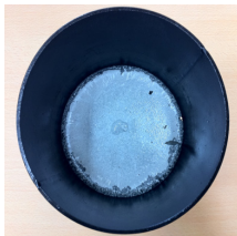
Fig. 3. Transported salt in a mold vessel.
