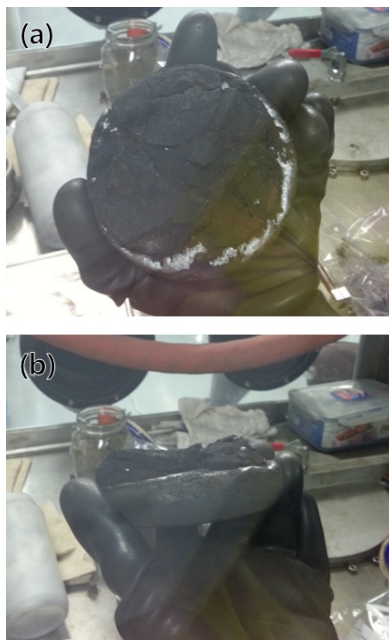
Fig. 2. Obtained U-ingot after melting test.
