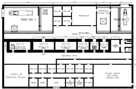
Fig. 2. General Arrangement for the Monitoring Building.
