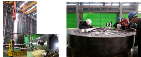
Fig. 14. Load test. Fig. 15. Hydrostatic test.
