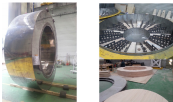
Fig. 9. Impact limiter and woods stacking.
