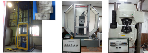
Fig. 11. Drop weight and impact tests.
