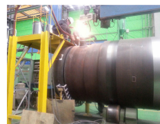
Fig. 5. Cask body welding.
