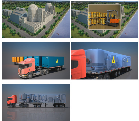
Fig. 3. The schematic diagram of the movable radio-active waste treatment apparatus.
