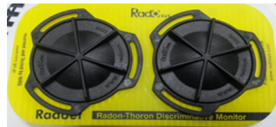
Fig. 2. Raduet passive-type detector.
