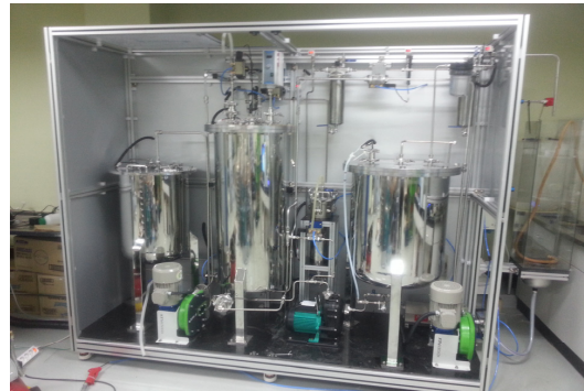
Fig. 1. Ultrasonic Waste Resin Treatment System.
