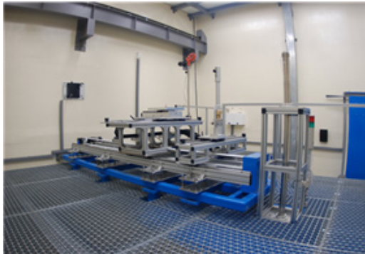
Fig. 1. CRI's ^{252}\text{Cf} Irradiator.
