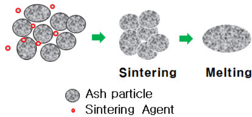
Fig. 1. Model for immobilization process of ash and sintering agent mixture.
