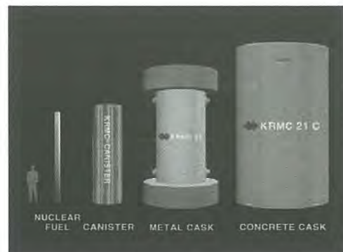
Fig. 1. Conceptual dwg of SF transport/ storage system.
