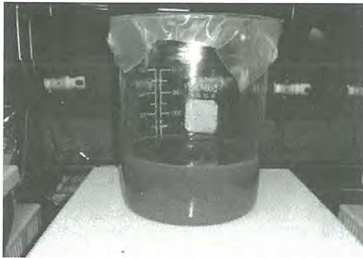
Fig. 2. Mixing Radioactive Waste Lubricant and Precipitant.
