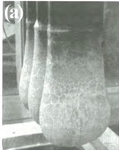
Fig. 2. (a) LiCl crystal image before sweating, (b) LiCl crystal image after sweating, (c) Separation efficiency of Cs, Sr and Ba from LiCl after crystallization and after sweating process.
