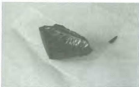
Fig. 2. Bulk Nd metal. Surface is easily oxidized, therefore shiny metallic portion was used for dissolution.
