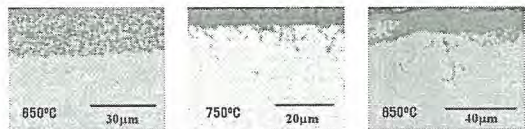
Fig. 2. Cross-sectional SEM images of Haynes 263 specimen corroded for 72 h. Region exposed to gas.
