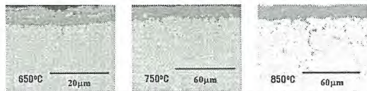
Fig. 3. Cross-sectional SEM images of Inconel 600 specimen corroded for 72 h. Region exposed to molten salt.
