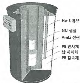
Fig. 1. Active neutron counter loaded an Am-Li neutron source and natural uranium oxide powder sample
