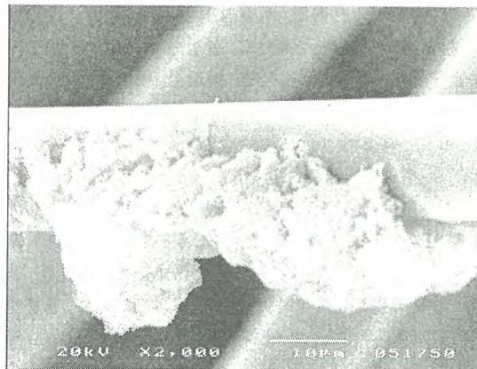
Fig. 3. SEM of Pd on the ACF Surface
