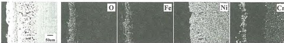
Fig. 3. SEM cross sectional image and elemental distribution of Haynes 75 corroded at 650°C for 168 hrs.
